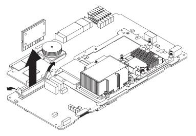
To replace the processor-board VRM, complete the following steps:
